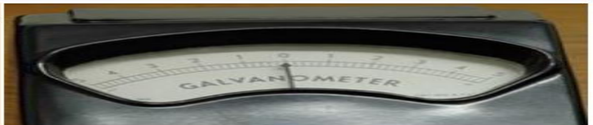
Schematic and photograph of a Galvanometer used for sensing electrical currents
